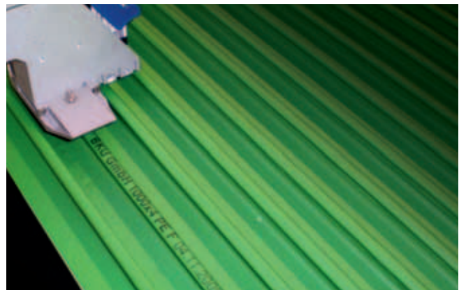
Coding of plastic profile plates
