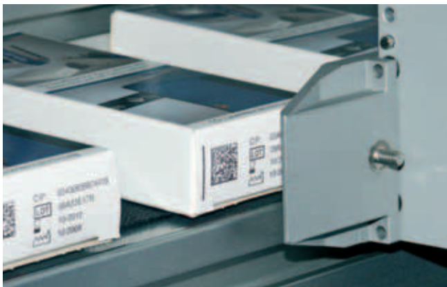
Cardboard box coding using DataMatrix code
